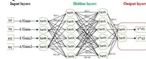
Figure 1: Neural network design with 2 hidden layers of 6 nodes each and 2 output nodes
