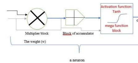
Figure 2 : Artificial neuron schematic design
