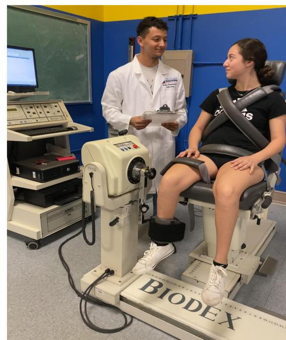
Figure 1: Biodex Dynamometer (not actual participant pictured)
