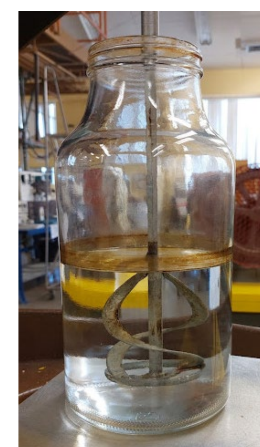
Fig. 7: left, DE test in which large amounts of the oil-dispersant solution are clinging onto the flask
