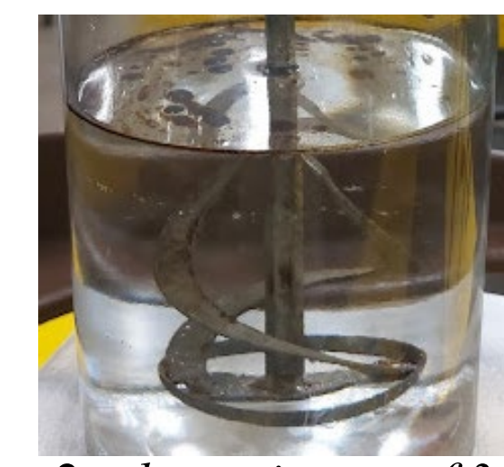
Fig. 1: above: image of 2.5-in. slanted turbine paddle impeller
