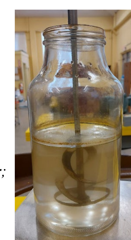
Fig. 8: right, DE test where flask was treated with an oleophobic coating prior; small amounts of oil-dispersant solution still clinging to flask
