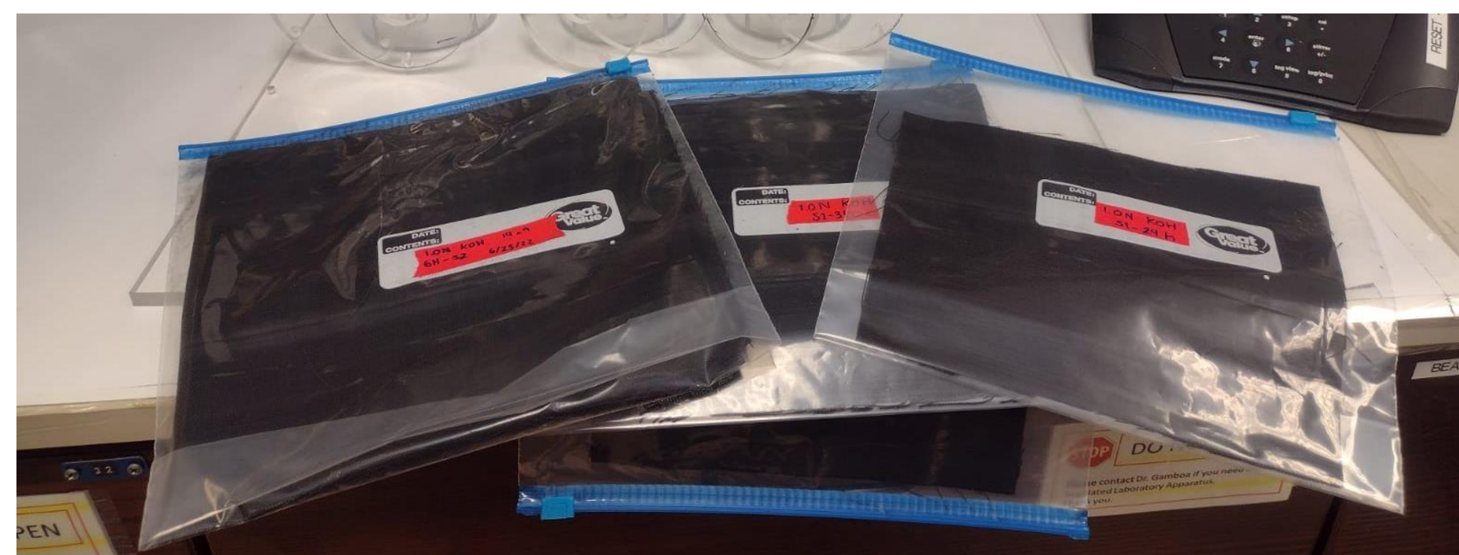
Figure 4. Examples of single waved activated carbon fiber cloth chemically impregnated with KOH at 3, 6, and 16h respectively
