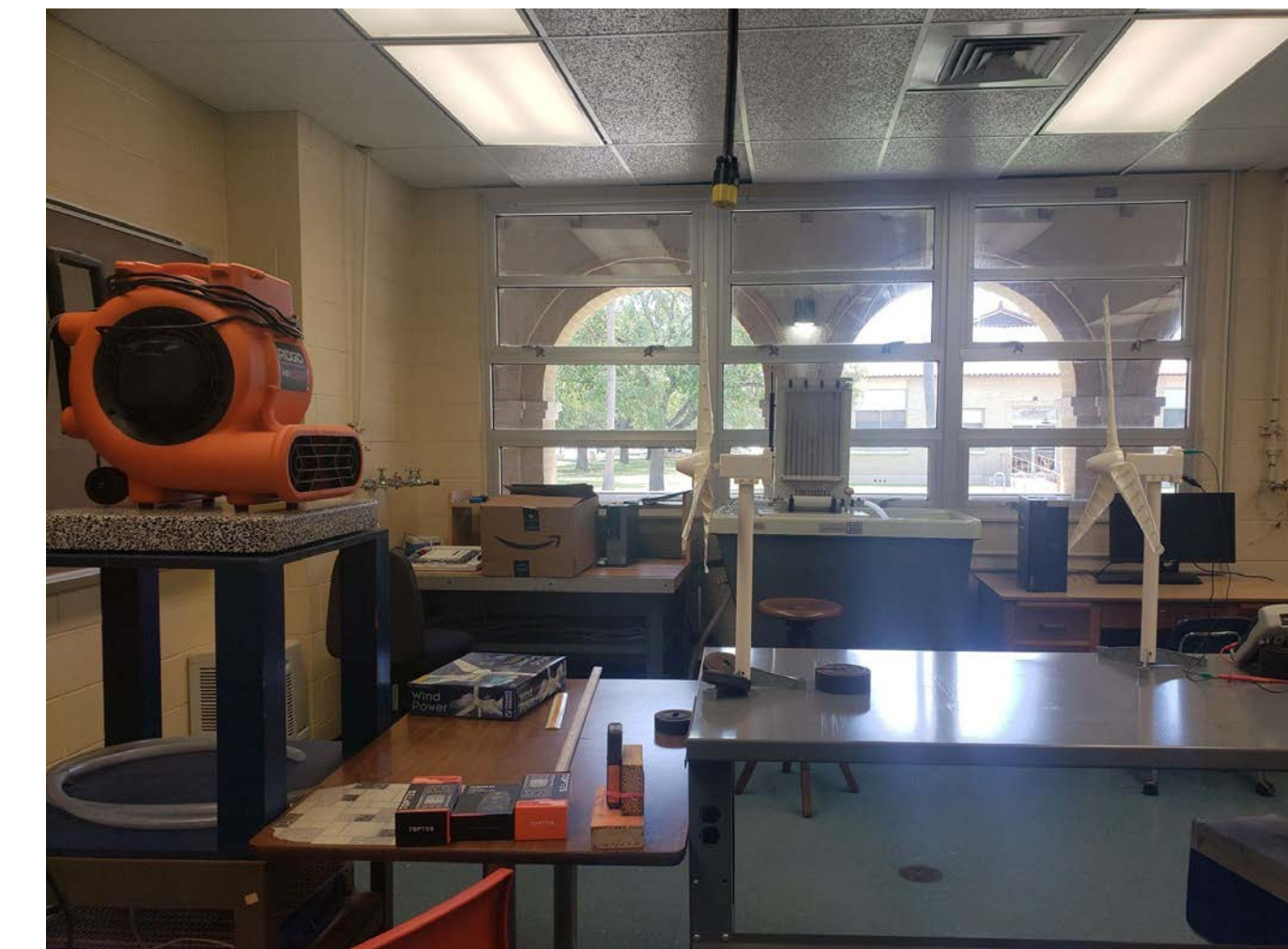
Figure 5: Side view of experimental setup. Distance from blower to fan is 31 inches. Fan spacing depicted is 36 inches horizontally.
