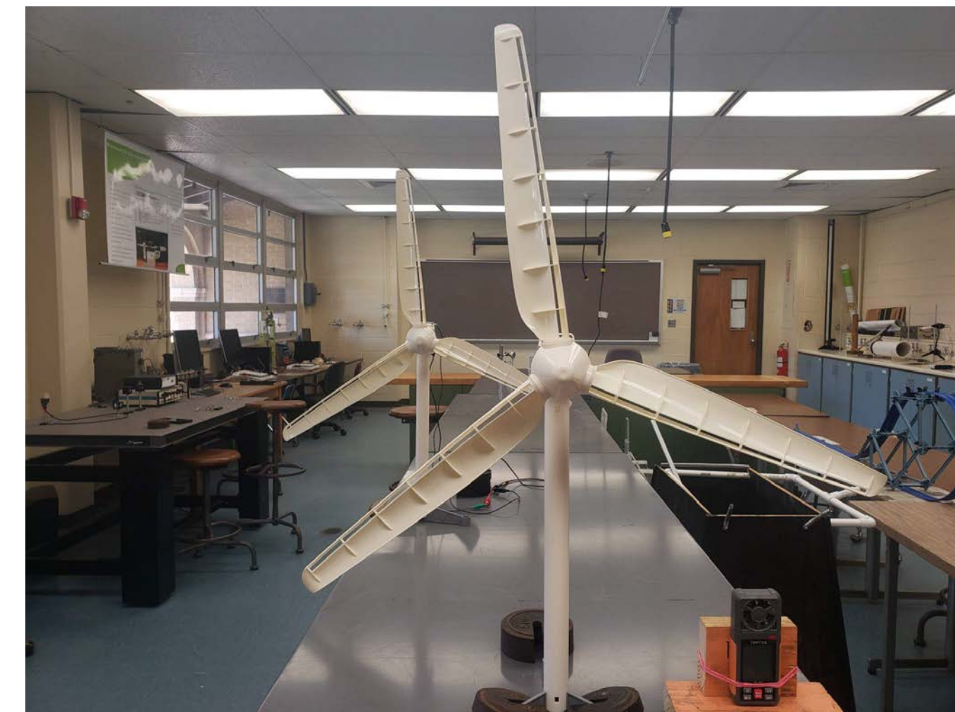
Figure 4: Frontal view of turbine 'b' in the wake of turbine 'a' while collecting voltage data. Fan towers offset by 10 inches.
