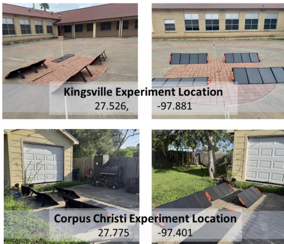
Figure 4: Solar panel test setups at Kingsville (top) and Corpus Christi (bottom) for irradiance comparison.
