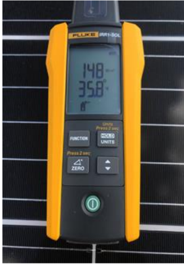
Figure 4: Fluke IRR1 Solar Irradiance Meter showing a sample reading for ETR and temperature.
