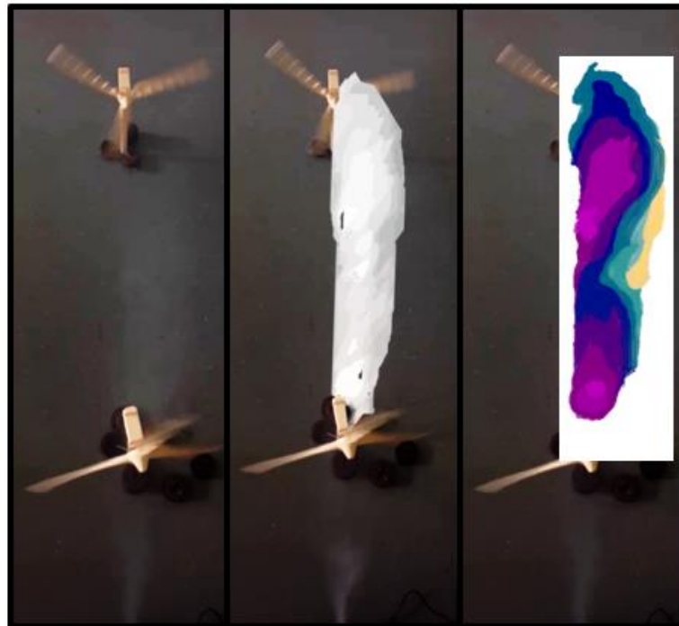
Figure 9: Aerial view of fog machine used to determine air travel. Picture on the left is the original image. Central and image to right show the enhanced images. The image at the right shows where speed is traveling at its fastest (purple color). The yellow color indicates wind traveling at a slower speed.
