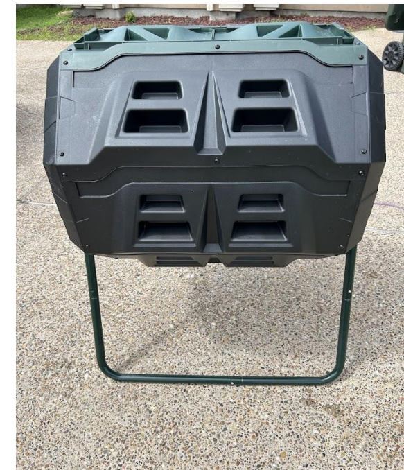
Figure 5: Assembled 43-gallon compost tumbler used for Bins B and C in the anaerobic composting experiment.
