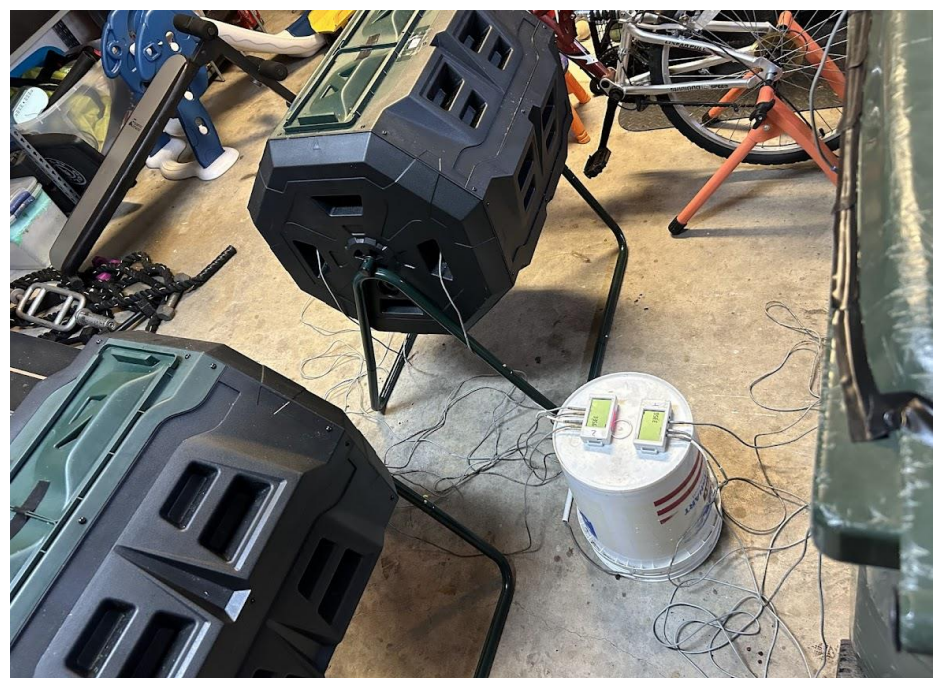
Figure 9: The figure depicts the orientation of all bins, sensor wires, and loggers in the garage environment, with the garage remaining closed throughout the duration of the experiment.
