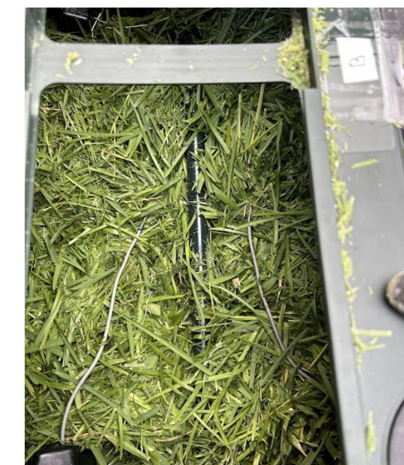
Figure 7: Temperature sensor placement in Bin B with grass at the midpoint of the biomass material. The figure shows the locations of temperature sensors inserted on the left and right sides of the compost tumbler.
