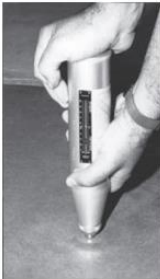
Figure 4: Rebound hammer test
