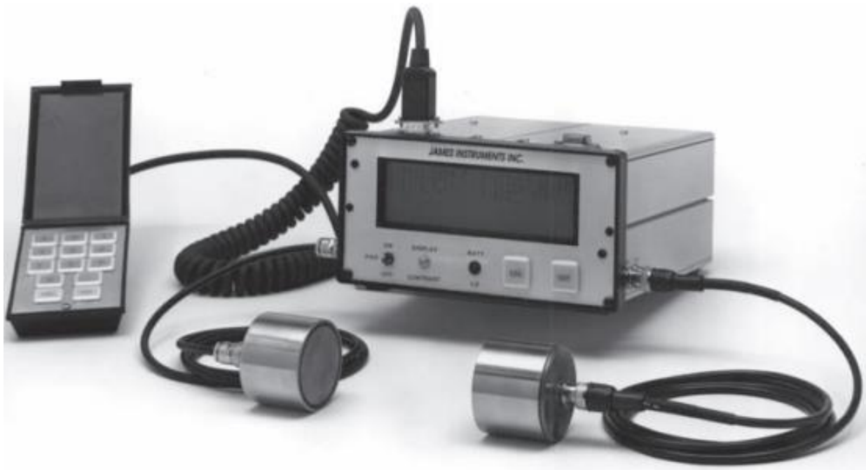
Figure 5: Ultrasonic pulse velocity test apparatus
