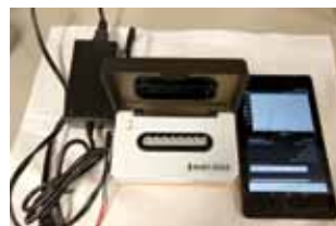
Portable device (Bio Ranger) connected to a tablet through Bluetooth
