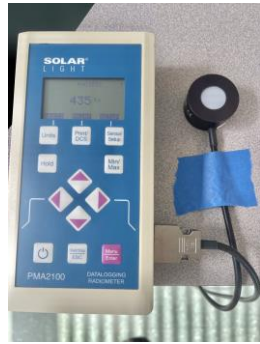
PMA2100 Dual-Input Data Logging Radiometer
