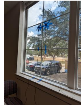
Photometric Sensor and Pyranometers secured to East window
