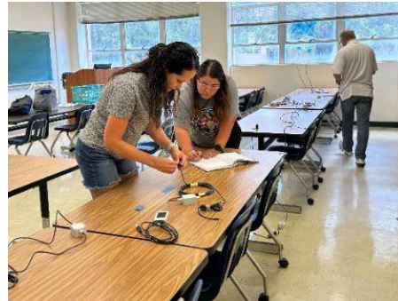
Securing Photometric Sensor and Amplifiers to desk surface
