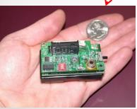
Spatially distributed sensors to *monitor* physical/environmental conditions (temperature, sound, pressure, motion, CO<sub>2</sub>)
